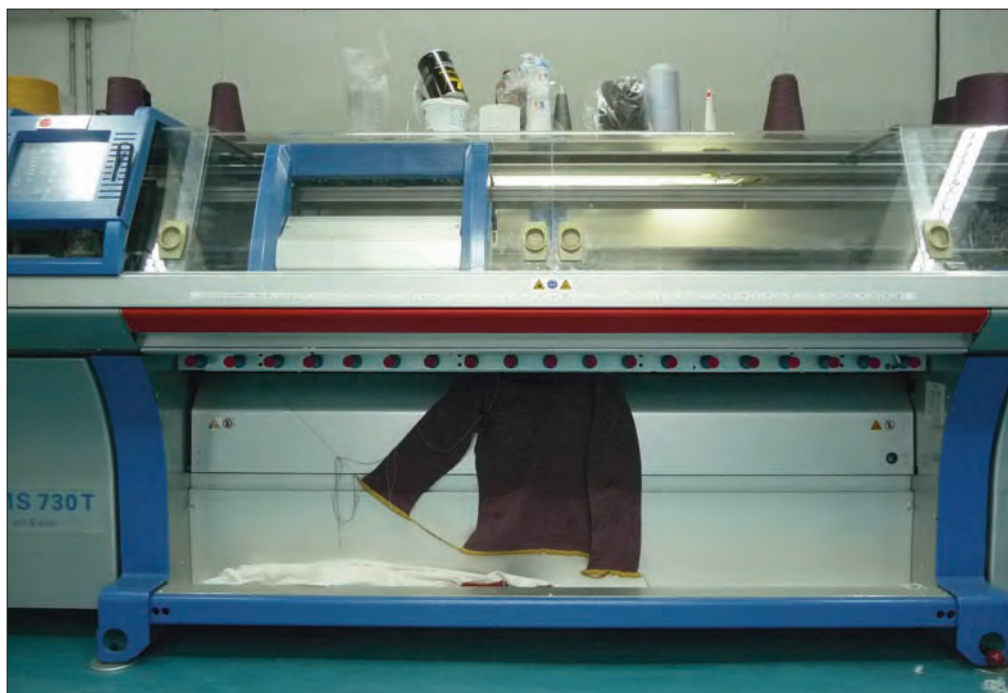
One step knitting process of seamless sweater (Photo: Sandy Black)
