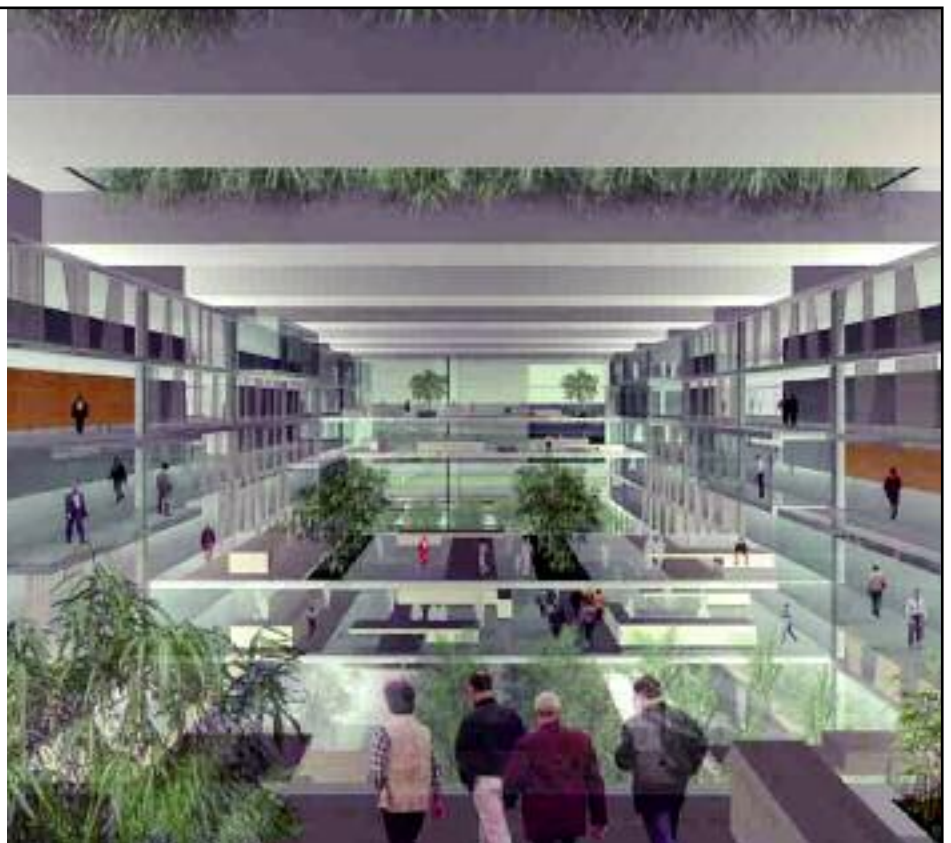
Figure 1: The heart of Amazon Court is a large, south-facing buffer atrium – a seven-storey tall, 32-metre wide public space which opens itself towards the sky
