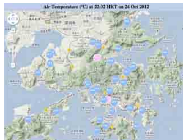
▲ Figure 3. Display of air temperatures on the Co-WIN webpage (data from an amateur observer is shown in the pink circle). Other weather elements include: relative humidity, maximum and minimum temperatures, wind speed, air pressure, rainfall, global solar radiation, ultraviolet radiation.
