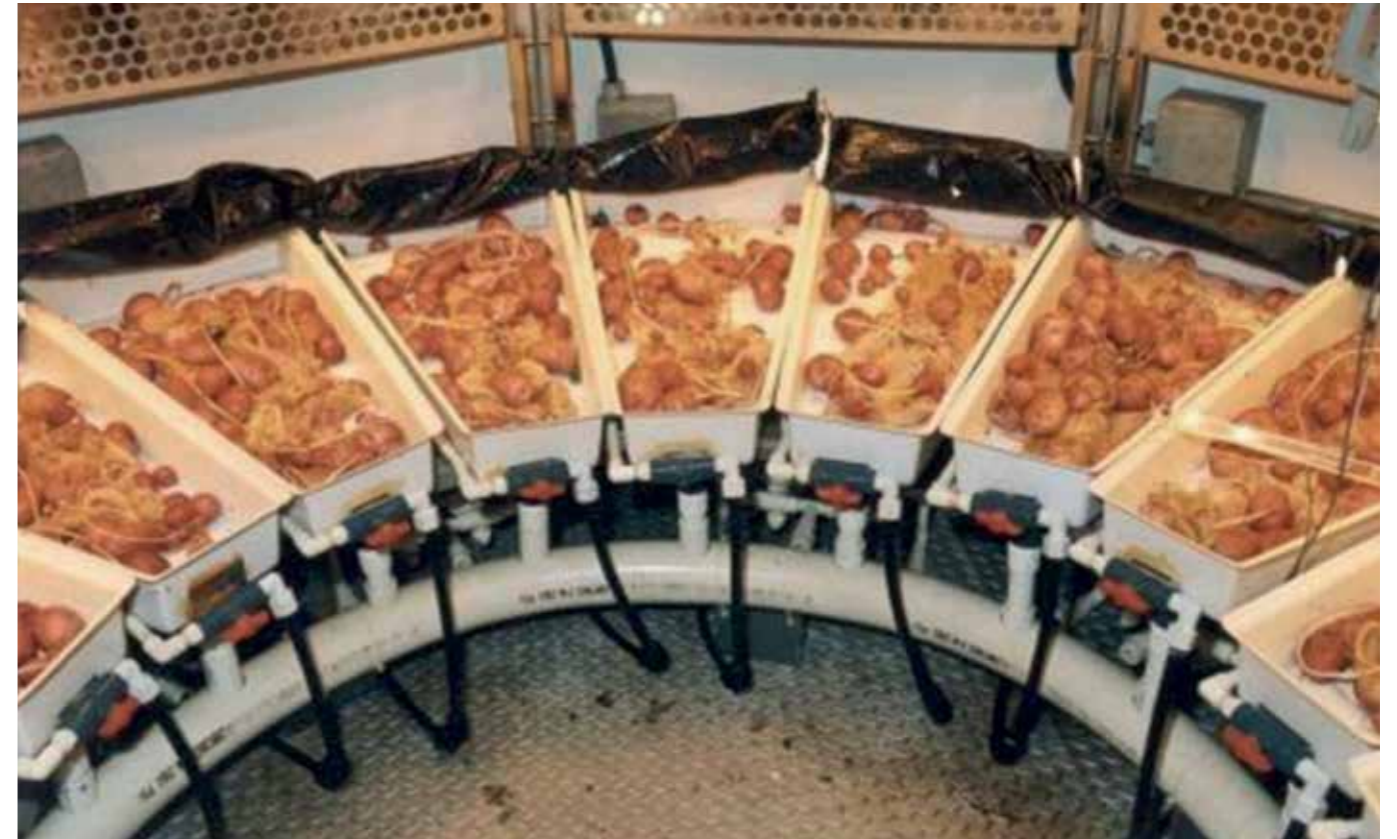
▲ Figure 2. Hydroponically grown potatoes were maintained for 105 days under electric lights in the Biomass Production Chamber at NASA's Kennedy Space Center. (Courtesy of NASA)
