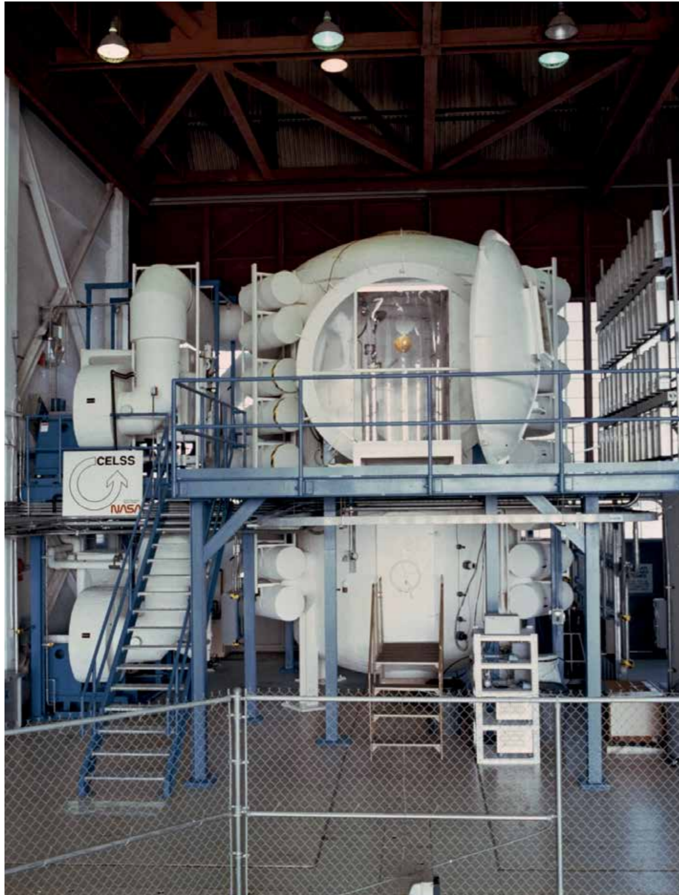
▲ Figure 1. The Biomass Production Chamber at NASA's John F. Kennedy Space Center. (Courtesy of NASA)
