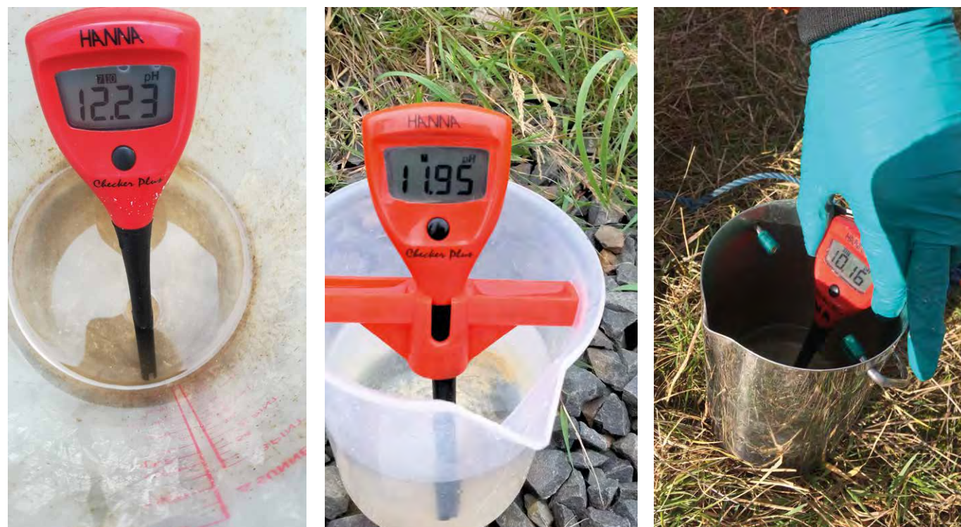
▲ Figure 2. Photographs of typical field pH measurements from site drainage that has been affected by alkaline materials. (© SLR Consulting Ltd)
