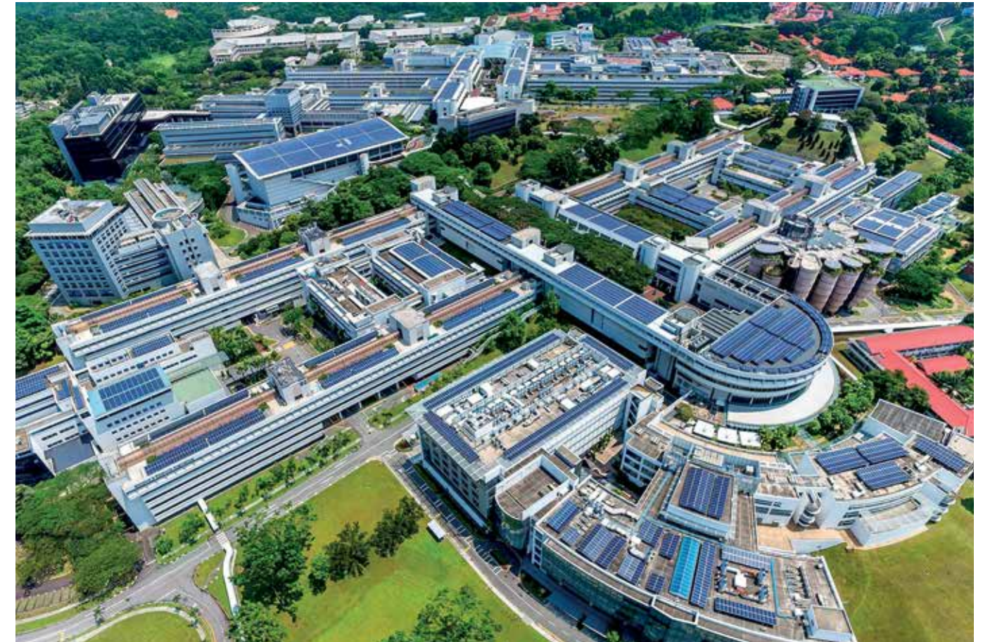
▲ Figure 6. Image of the 5,000 kW rooftop solar photovoltaic installation at NTU Singapore campus (© Nanyang Technological University Singapore).
