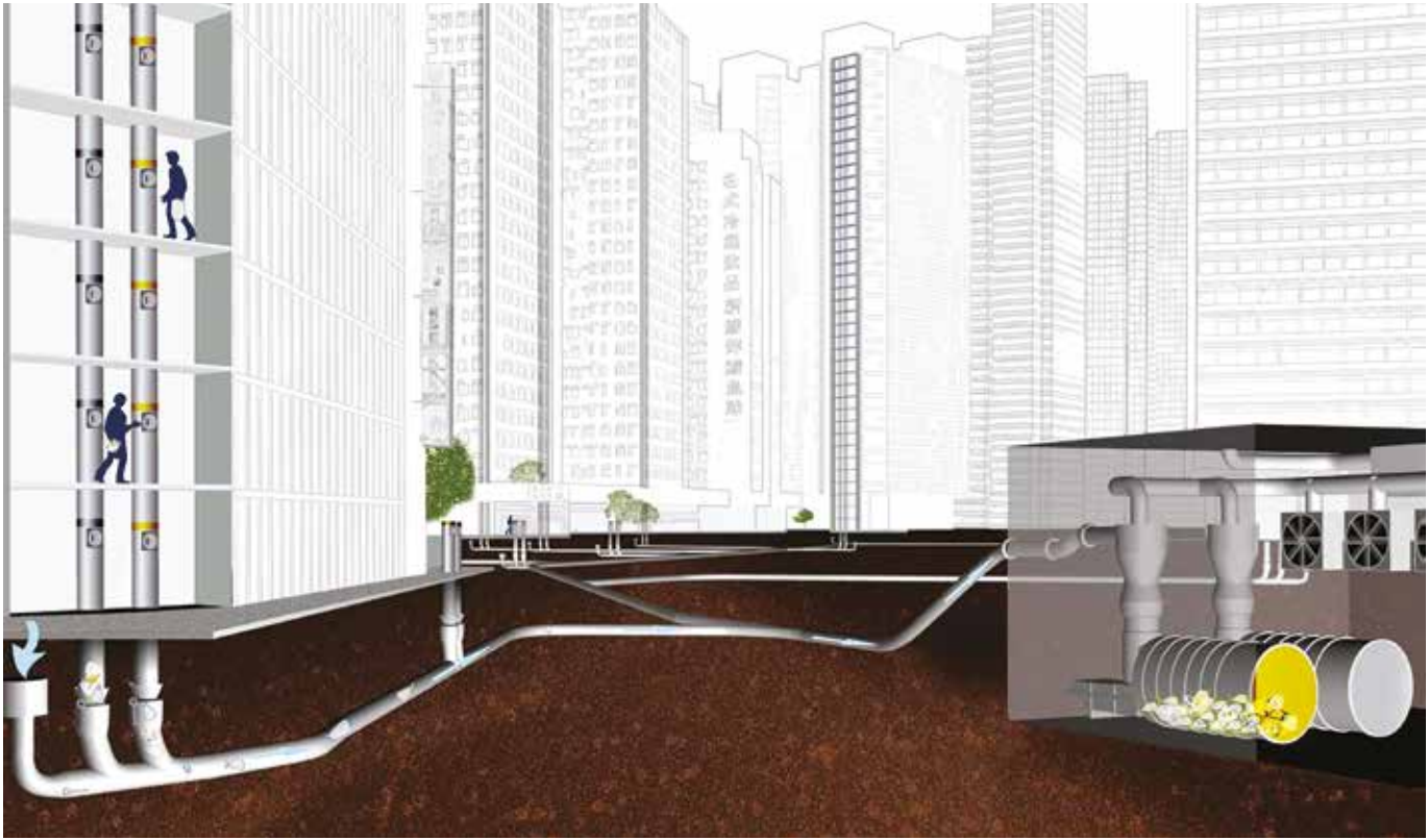
▲ Figure 3. The pneumatic waste conveyance systems (PWCS) used in Singapore. (© Envac)
