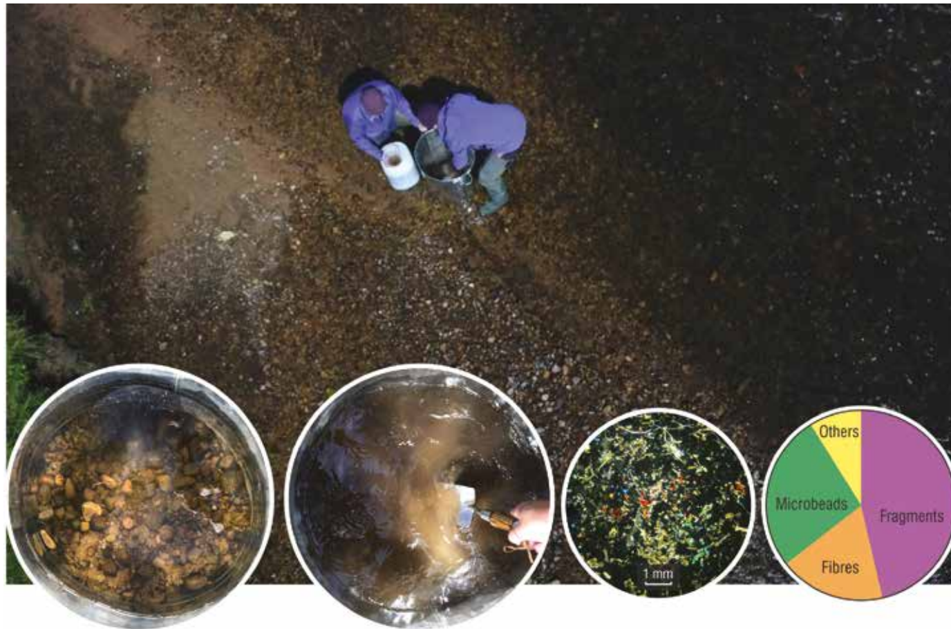
▲ Figure 3. Sampling microplastics stored on the channel bed under low-flow conditions. Microplastics are present within the sandy and silty sediments between the loose gravels. The insets summarise, from left to right, the field sampling and laboratory recovery of microplastic particles. A known area of channel bed is isolated using the aluminium cylinder, the gravels are agitated to bring the fine sediment load into suspension, samples of turbid water are returned to the laboratory where the recovery, identification and quantification of microplastic particle types takes place. This sampling method also allows us to estimate the amount of fine sediment stored within and on the channel bed. (©Mike Wafer, Outpost Pictures, with graphics drawn by Nick Scarle, The University of Manchester)
