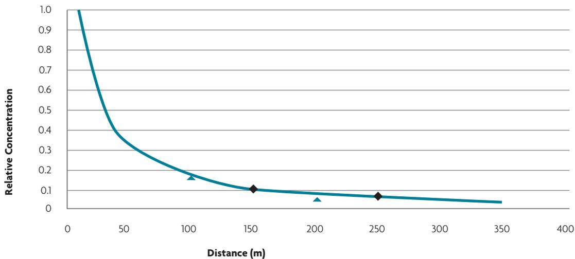
Also shown are data points from PM<sub>10</sub> Survey Around 'Worst Case' Coal Handling Plant. The data points were normalised to fit on the line at the nearest point to the source
