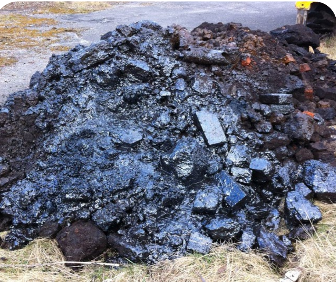
Made ground from remediation scheme at former oil refinery and vitriol works. Stoke-on-Trent, Staffordshire. © Stoke-on-Trent City Council
